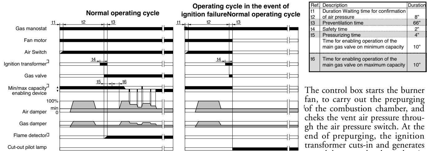
The same time the two gas valves open (Vs safety valve and Vl Low flame working valve). The total safety, in case of missed ignition or casual burner's flame-out, is granted by a ionisation probe which cuts-in and sets the burner shutdown within the safety time. In case of gas lack or a major pressure drop, the minimum air pressure switch shuts down the burner.
