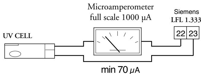
The detector current is checked by inserting a microammeter (scale 1000  $\mu\text{A}$  - d.c.) in series with the uv cell..
